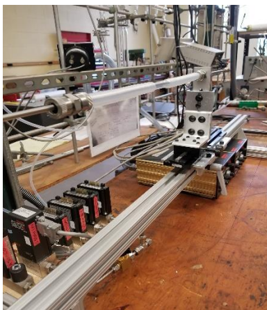
Figure 1. Photographs of the devices developed under this project. Left: tube coating device. Right: Small gas-surface reactor with movable injector
