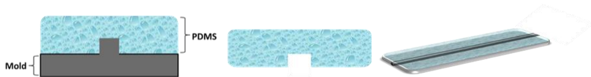
Figure 1- (left) A cross sectional view of the PDMS polymer (type of plastic) as it hardens on the mold. (middle) A cross sectional view of the completed channel. (right) A top view of what the completed microchannel would look like. The PDMS polymer cures with a thin channel running along it.
