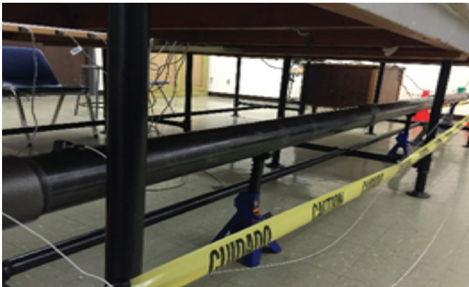
Advanced Communication and Signal Processing (aCASP) Lab testbed at NJIT for communication via steel pipes
