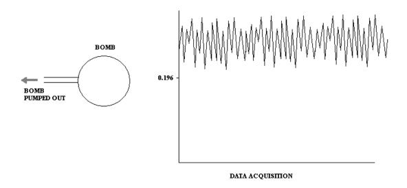
Start the data acquisition by pressing the spacebar. Turn the vacuum valve (VALVE 1) slowly toward the VESSEL (see panel diagram). Observe the trace approaching from top of the screen. Turn the VALVE 1 back to normal position to stop the trace at 0.196V, which corresponds to 4.87 psiA {calibrated to y=24.996x -0.0242}. Press the spacebar to stop data acquisition and close the vessel valve.
