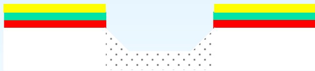
Boron Implantation of Silicon
