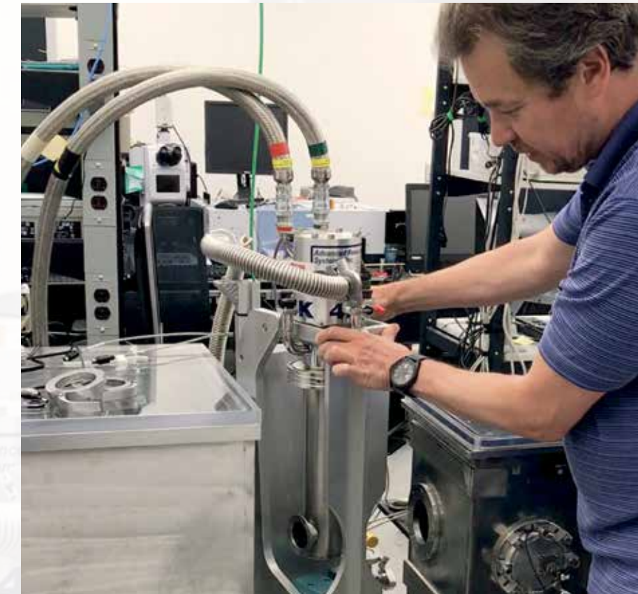
At his beamline station at Brookhaven National Laboratory, Andrei Sirenko uses an ellipsometer, which shines synchrotron radiation on the material to analyze polarization of the reflected light, thus revealing unique material properties in the THz spectral range.
