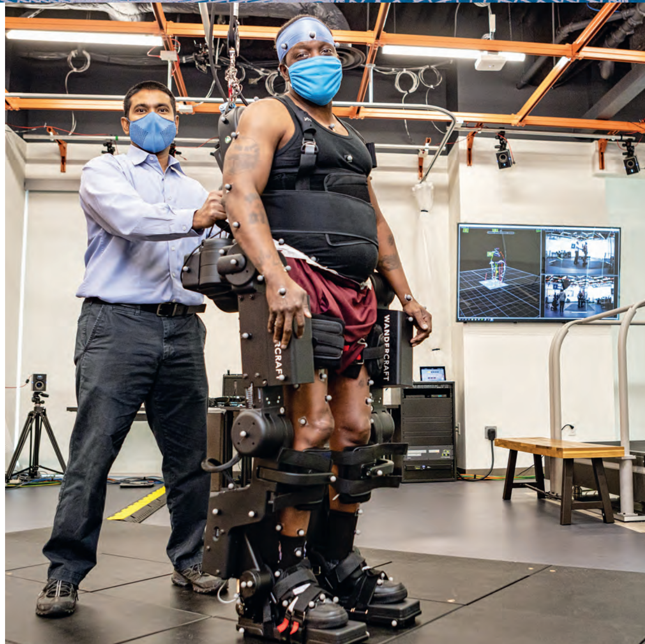
Damyane Evely, a paraplegic, was the first person in the U.S. with a spinal cord injury to test a new, self-balancing exoskeleton with 12 degrees of freedom that is designed to more closely approximate human gaits than current models. He took 1,100 closely observed steps that day in Saikat Pal's Life Sciences Motion Capture Laboratory.
