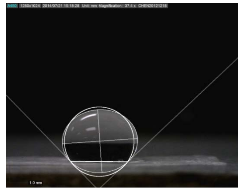
Contact Angle on Polyvinylidene fluoride scaffold
