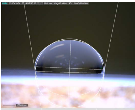
Contact Angle on Teflon Film
