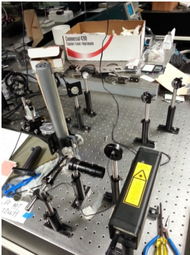
Left: The mirrors and beam splitter set up to make the lasers incident on the prism's surface.
