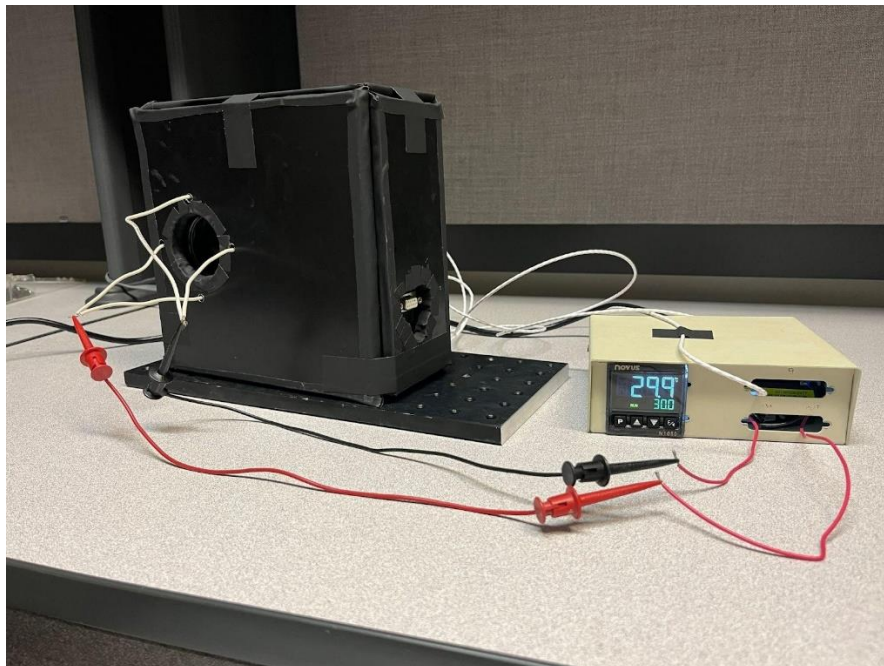
Figure 1: Thermal controlled filter wheel system including the filter wheel box (left) and PID temperature controller box (right)
