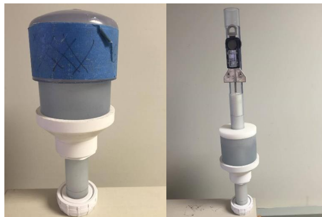
Figure 1: Apparatus for the new method to measure fines
