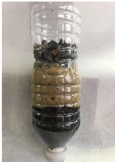
Figure 1: Inexpensive water filter made of biochar for removing heavy metals.
