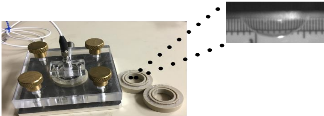
Figure 1: Blasting device highlighting well expansion after blast
