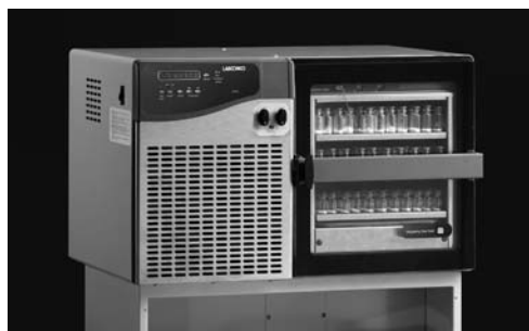
Batch drying in a tray dryer permits precise control of product temperature and heat input.
