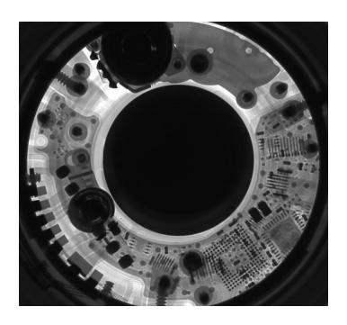
**Photo:** A Canon DSLR Lens (24mm f2.8 pancake lens) is imaged at resolution of ~20 micron using a Bruker SkyScan microCT scanner. The camera's outside ring is composed of thin metal, while the darker inner circle of the camera lens is composed of dense glass. Credit — Mathew Schwartz/NJIT
